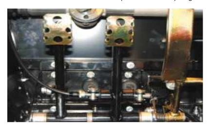
The position of the pedals can also be adjusted by **a)** adjusting the pedal face, **b)** adjusting the pedal angle and **c)** by moving the pedal pivot shaft. **PLEASE NOTE** that **c)** will require changing the master cylinder push-rods which are available online.
