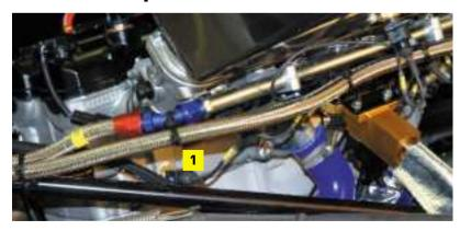
1 ECU coolant temperature sensor
